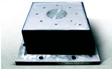
The isolation bearing system works by lengthening the fundamental period of the structure, thereby reducing the acceleration input into the building, bridge or equipment. The damping
